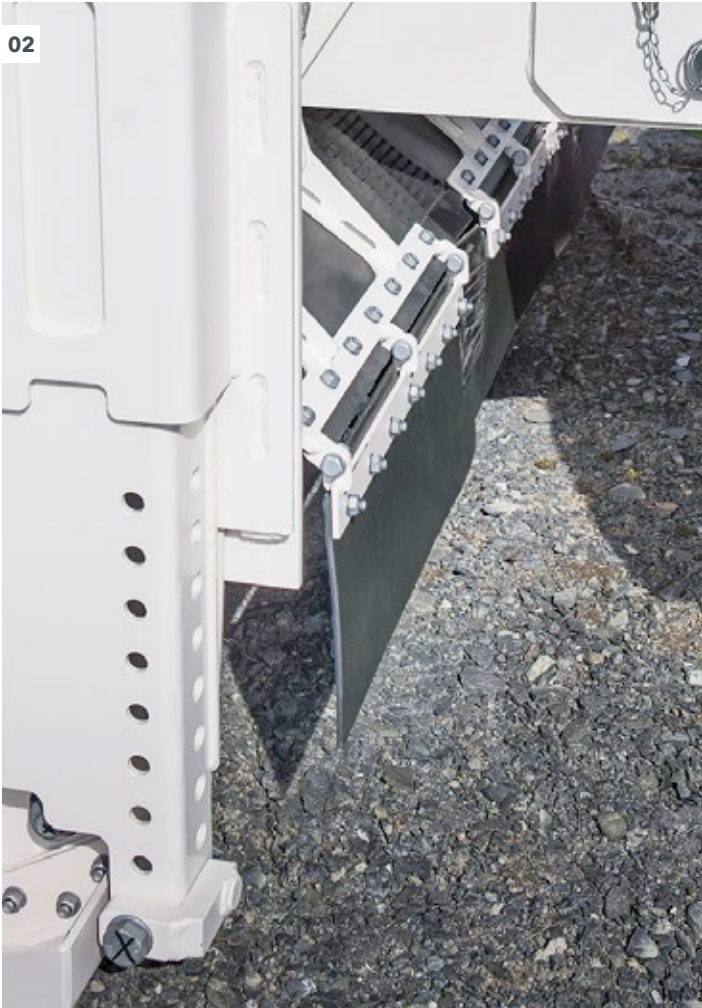
01 The stone guard is proving its worth in operation: no flying stones and less dust.
