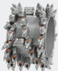
Standard Milling Drum Milling width: 600 mm Milling depth: 0 - 280 mm Tool spacing: 12 mm
