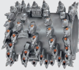
Standard milling drum Milling width: 1,000 mm Milling depth: 0 - 330 mm Tool spacing: 15 mm
