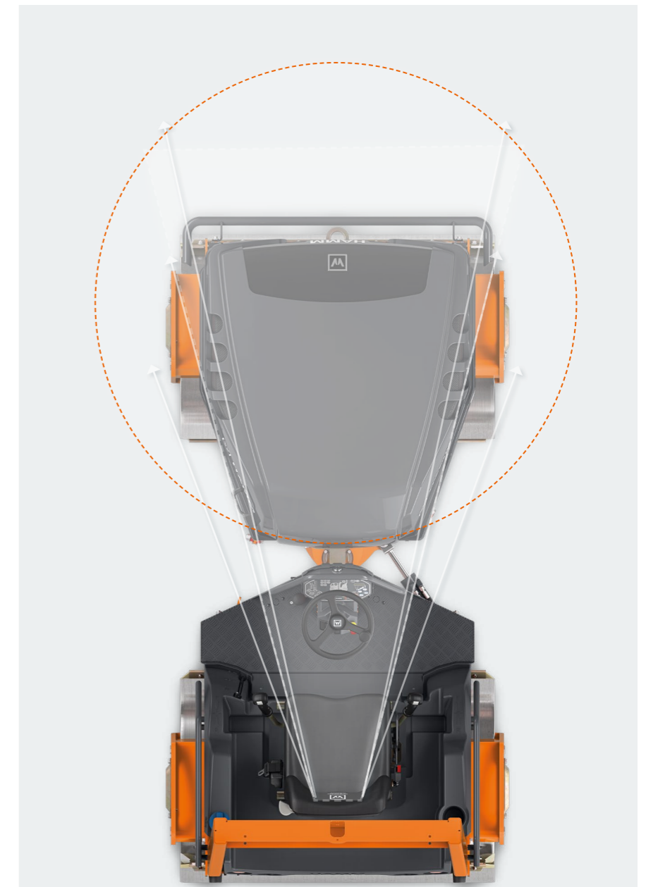
Elevated side plates provide plenty of side clearance when working alongside kerb edges.
