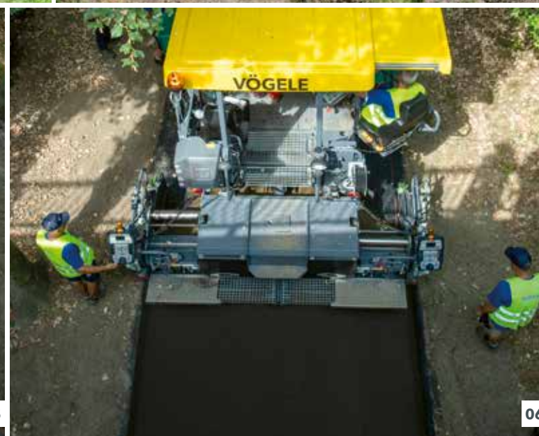
04 The paver operator's platform ensures maximum visibility. 05 Large material hopper for optimum feeding with mix. 06 AB 340 Extending Screed ensures a perfect paving result.
