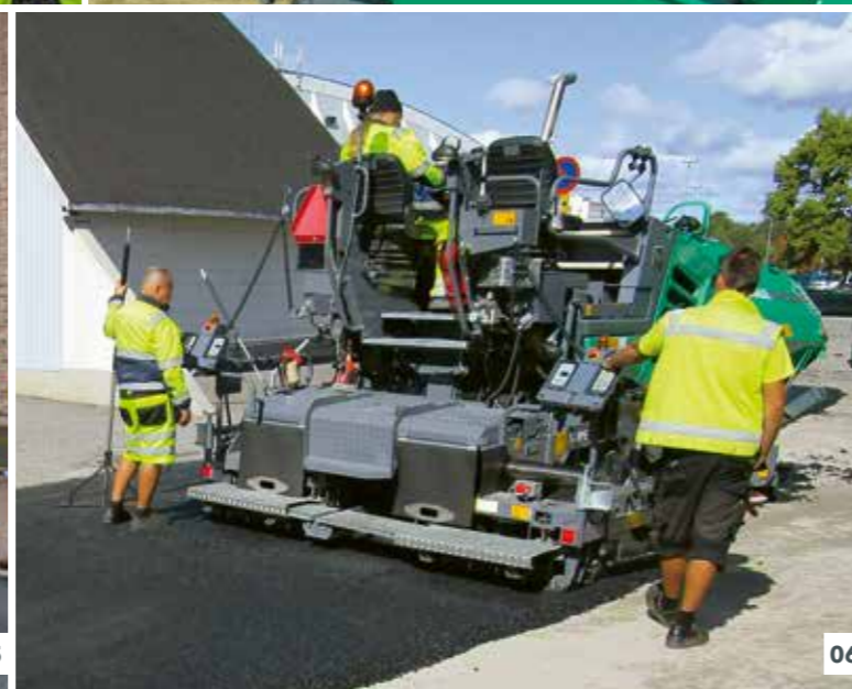
04 The paver operator's platform ensures maximum visibility. 05 Optimum feeding with mix thanks to the large material hopper. 06 Can be combined with the AB 340 Extending Screenshot.
