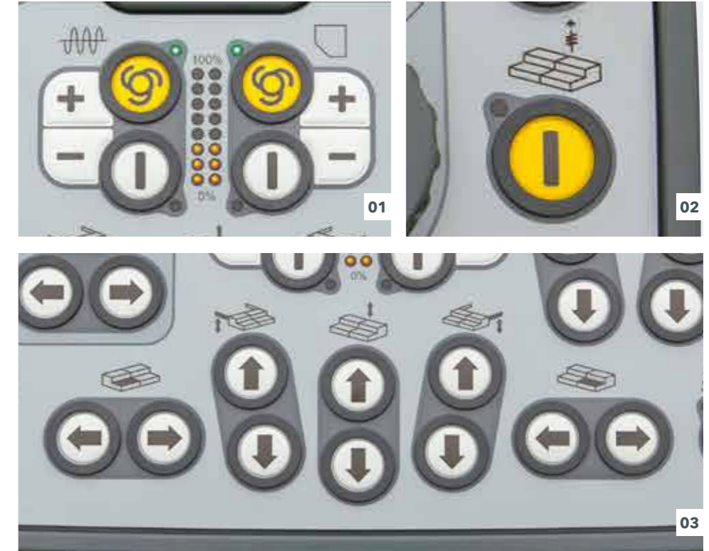
01 Precompaction performance 02 Screed Assist (option) 03 Screed settings
