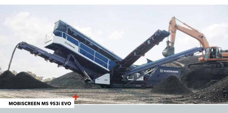
The mobile screening plant MOBISCREEN MS 953i EVO is equipped with a 102 ft squared screen box. The triple-deck screening plant impresses with a feed capacity of up to 551 US t/h. It is controlled using a modern control system. As a result, all functions are easy to control and operating statuses and machine functions can be viewed at any time.
