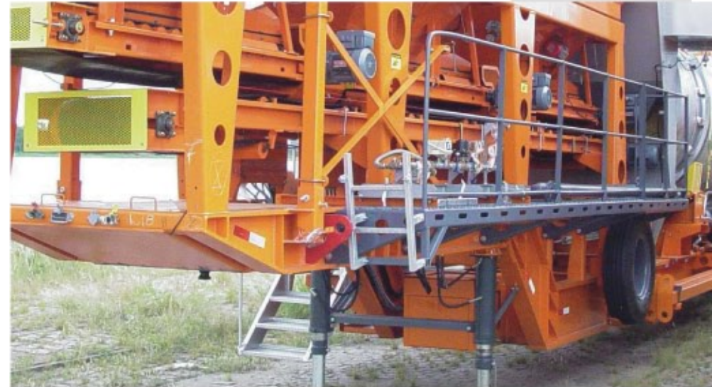
Inspection Platform for the Bins
