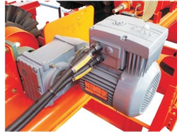
The gear motor has a coupled frequency converter.
