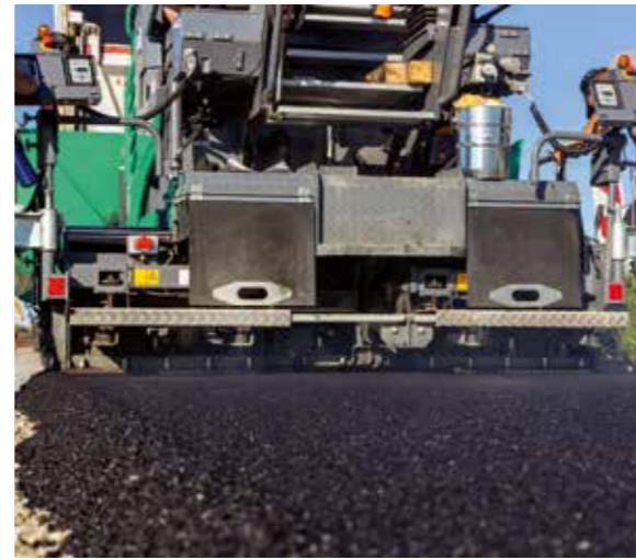
AB 340 Extending Screed with 25 cm bolt-on extensions
