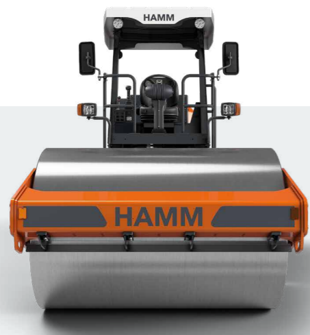
Plastic protective roof
