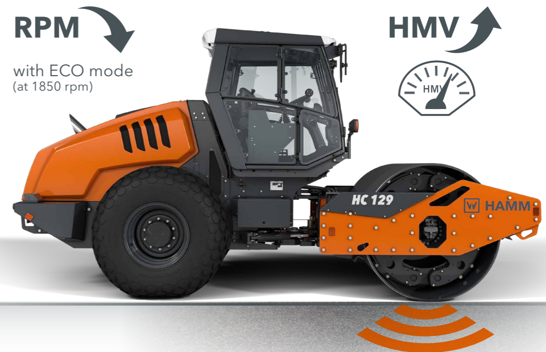
In ECO mode, the compactors work at a reduced speed of 1850 rpm. The compaction power stays consistently high.
