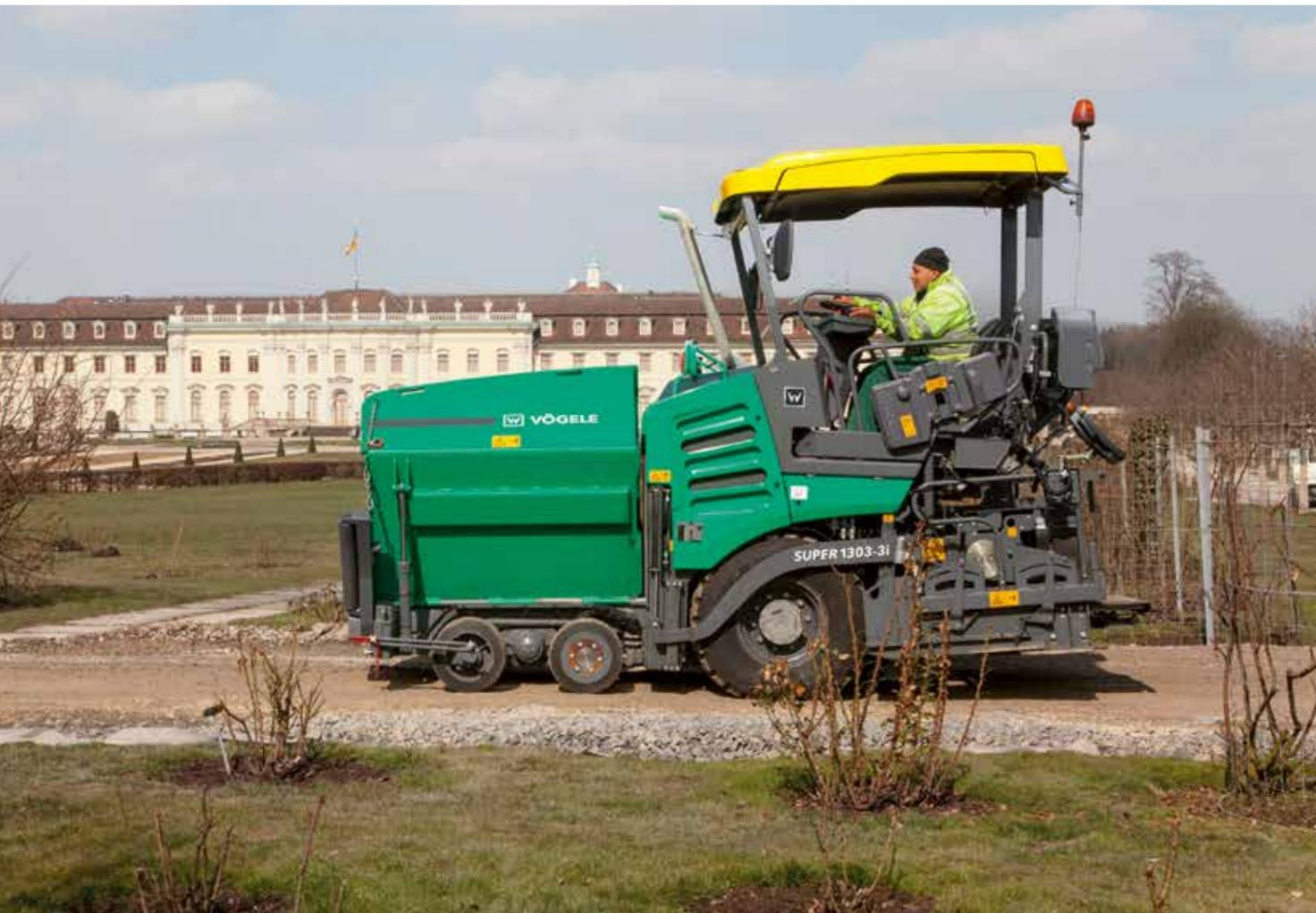
The separate hydraulic drives in both rear wheels and two front wheels ensure maximum power transmission. Electronic Traction Management and an electronically limited slip differential acting on the drives of the rear wheels assure optimum traction, even on difficult terrain.
