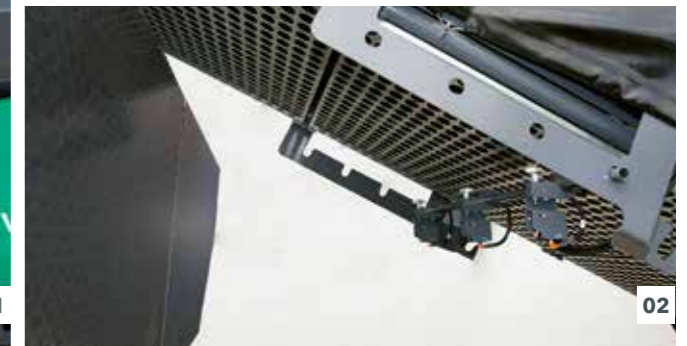
01 Mechanical distance control is also available for the MT 3000-3(i) Standard as an alternative to laser-controlled distance control. 02 Laser-controlled distance control for VÖGELE PowerFeeders consists of three individual laser sensors.
