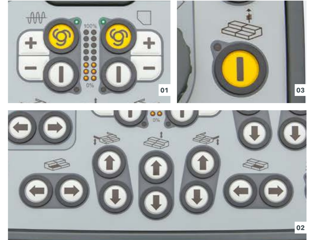
01 Precompaction performance 02 Screed settings 03 Screed Assist (option)
