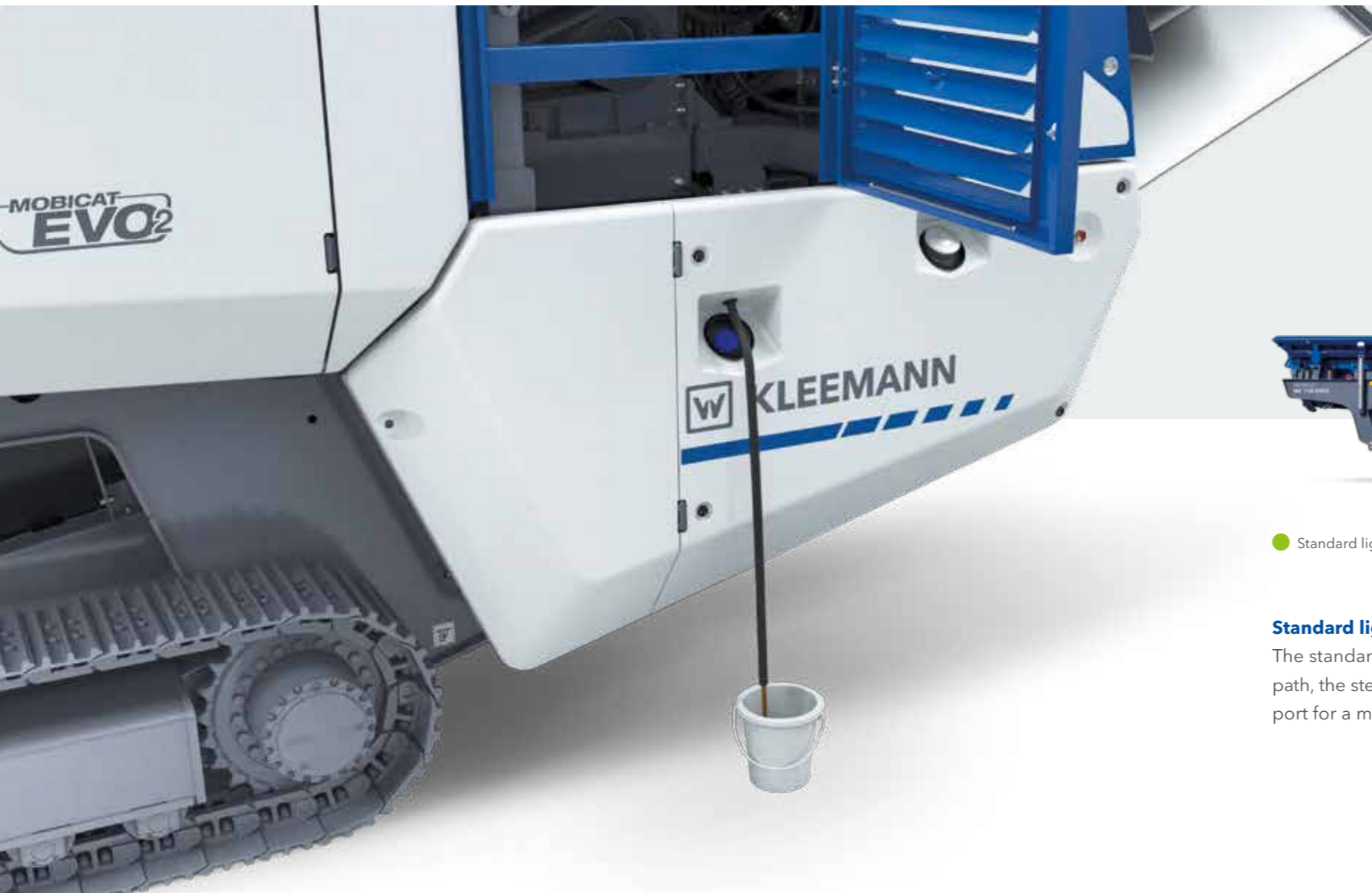
Central drain point
